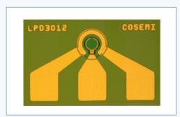
Cosemi's LPD3012 is a mesa-structured, InGaAs/InP-based PIN photodiode offering high responsivity, low dark current and low capacitance for high bandwidth, high performance optical receiver designs.
